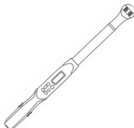
3/8" Calibrated Torque Wrench 5-100 ft/lbs.
